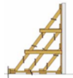
Figure 8 – Triple Raker shore [6]
