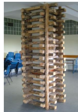
Figure 5 – Cribbing [Photos transferred by RSB]
