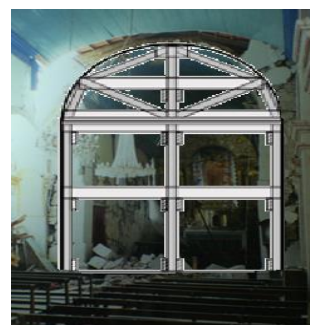
Figure 17 - Solution for shoring of arch
